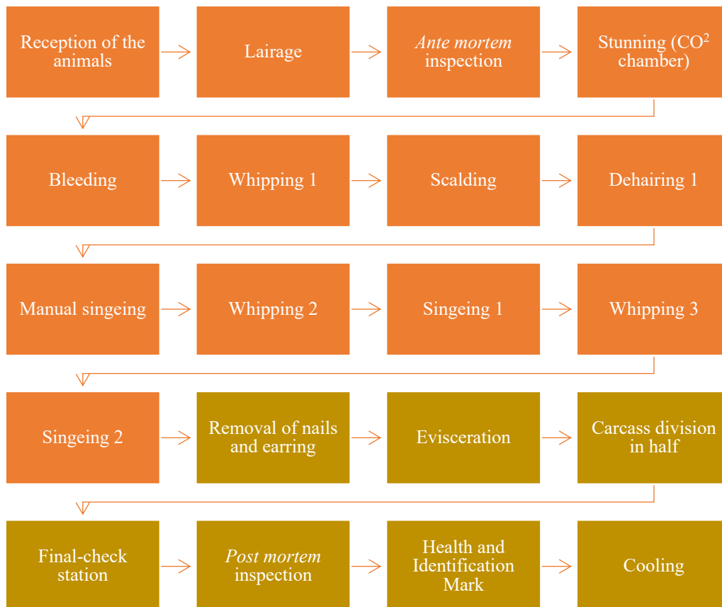
Figure 4 – Process of pig slaughtering process at the Spanish abattoir. Note: Orange – Dirty zone; Yellow - Clean zone.
